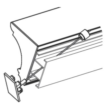
The Trim Maker extrusion and base are mounted to a Porsa extrusion. The graphic is inserted into spring clip holders. The spring clip holders are slid in through the end of the Porsa extrusion and the Porsa endcap is affixed. To change the graphic, remove the Porsa endcap, slide out the graphic and slide in the replacement.
